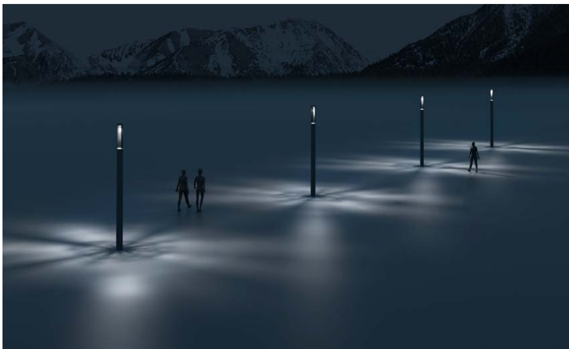
H.3100 mm Simulation performed with Screen 38W 3000K Optics 360° Wide Luminaires interdistance 12mt.
