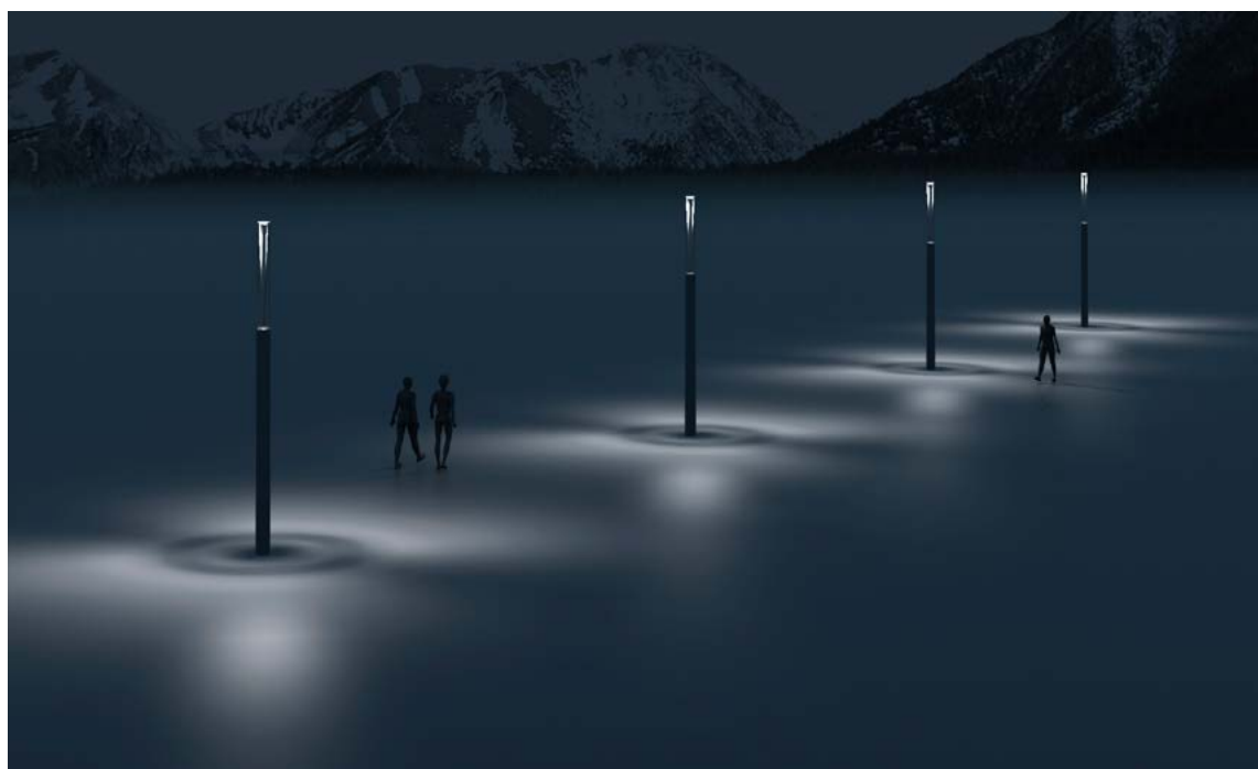
H.3700 mm Simulation performed with Rush 38W 3000K Optics 360° Luminaires interdistance 10mt.
