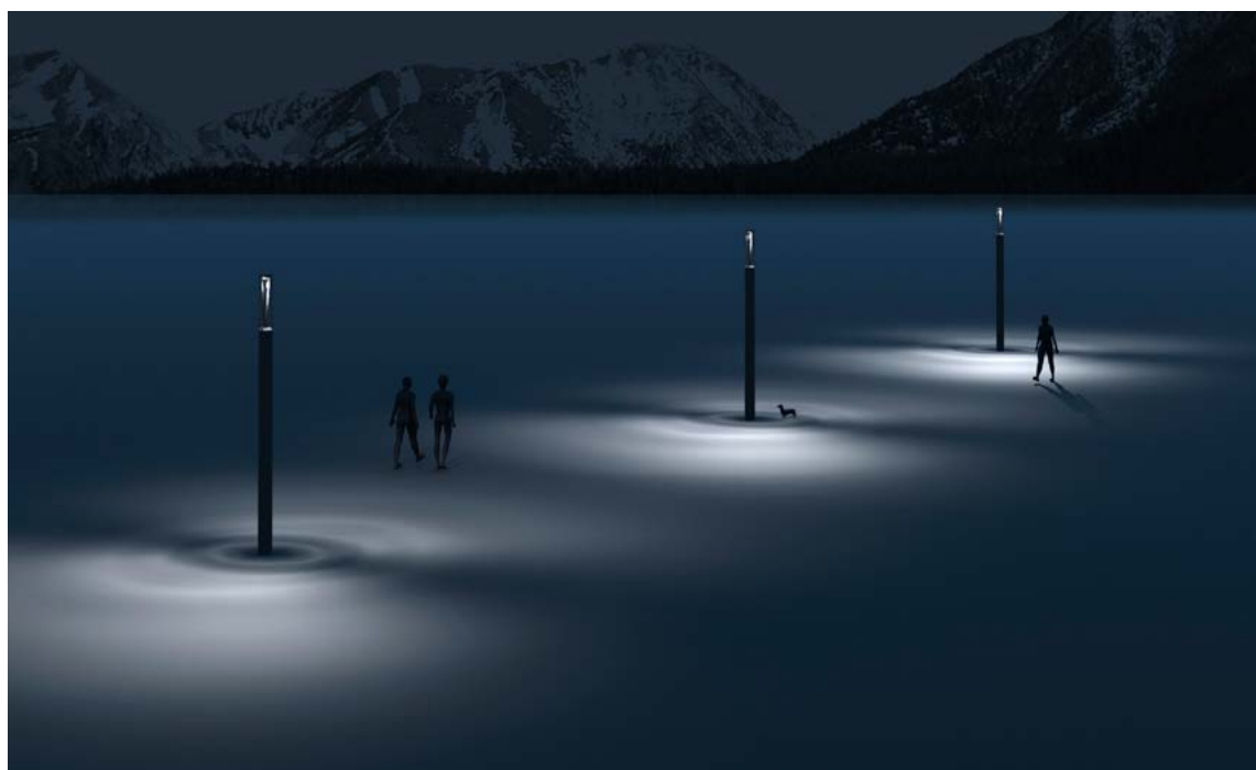
H.3100 mm Simulation performed with Rush 38W 3000K Optics 360° Wide Luminaires interdistance 12mt.
