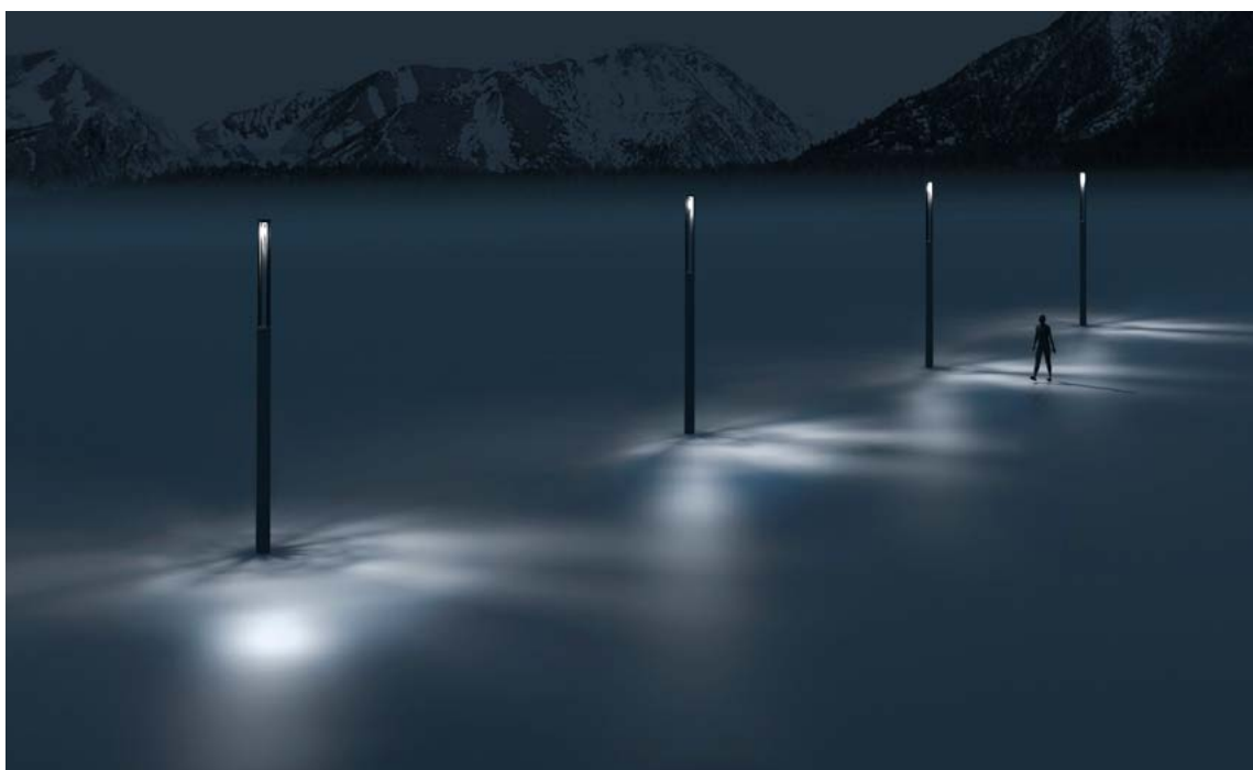
H.3700 mm Simulation performed with Screen 38W 3000K Optics 180° Luminaires interdistance 10mt.
